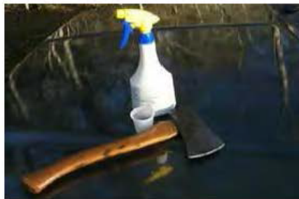
Application equipment: Chemical resistant spray bottle, metric dose cup for calibration of spray bottle, and hatchet.
